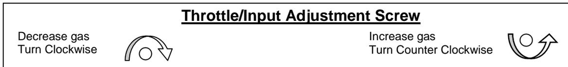
**Combustion Calibration** - To calibrate burner operation, perform the following procedure using a calibrated combustion analyzer capable of measuring CO<sub>2</sub> and CO from Natural and Propane Gas burning boilers:
