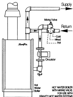
open between the "cold" and "mixed" ports, the "hot" port is closed, and the system is circulating normally, as if the valve were not there. Only it's flow resistance remains in the system, preventing the pump from overloading.
